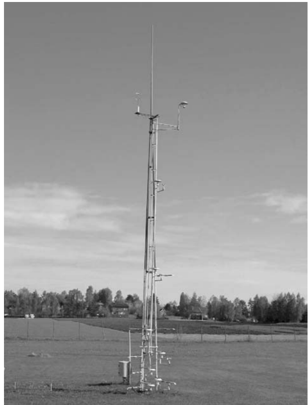
Fig. 4. Mast for profile measurements of temperature and wind
