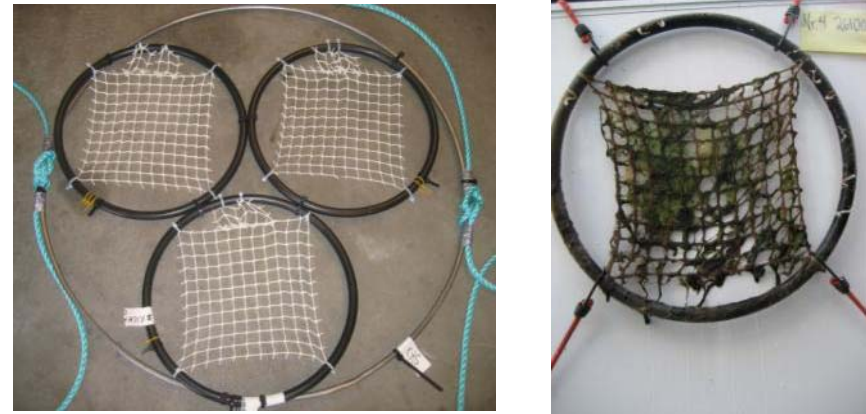
Field test systems for marine growth on fish farm nets (Photo T. Nordtug)
