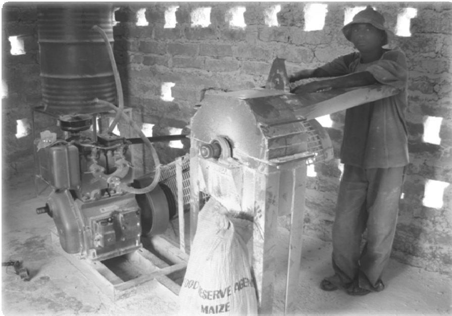
Figure 32: A hammer mill can run on pure jatropha oil
